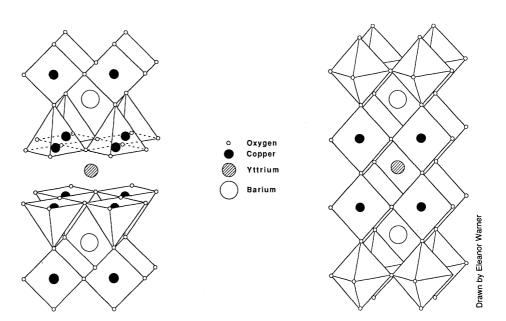
**Superconductor crystal structure.** (Left) The accepted crystal structure of the yttrium-barium-copper-oxygen superconductor is characterized by the absence of oxygen on the yttrium plane. Note that not all the copper atoms are visible. (Right) By moving the oxygen vacancies to the copper planes neighboring the yttrium, an alternative crystal structure with a more common mixture of octahedral and square planar coordinated copper atoms is generated.
