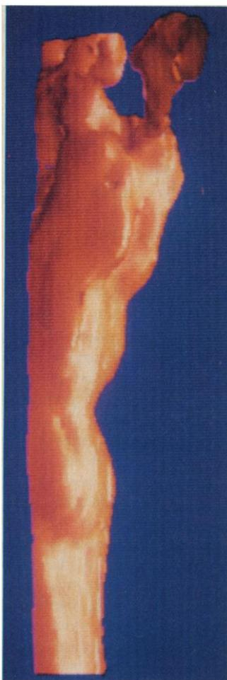
**Fig. 2.** Reconstructed constant concentration surface in the transitional region of a gas jet. The region shown is 6.8 by 2.1 by 0.7 nozzle diameters ( $d = 2$  mm) in dimension, centered at 10 diameters downstream of the nozzle orifice and with one side bisecting the upward flowing jet.
