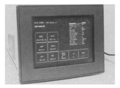
from the presented choices. The user responds by lightly touching one option. The 1021, acting as a software-configured control panel, then relays the choice to the computer. The touch screen may be mounted into a panel or rack or set on a tabletop. High-level software allows the user to design "touch targets" with only a few commands. ICS Computer Products. Circle 568.
