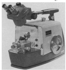
versal knife stage provides control without spring-loaded locks. The MT-2C features a stage-mounted block for accurate trimming. A fiber optic lighting system permits knife-to-block approach to within 20 nm, and a mechanical advance system advances the specimen in increments of 1 nm to 4 mm. RMC. Circle 545.
