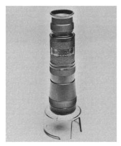
optics provide a bright image with ambient light in most situations, and field-usable lighting accessories are available for low light conditions. The macroscope may be adapted for use with a 35-mm single lens reflex camera for photomicrography at magnifications of  $\times 18$  to  $\times 36$ . It incorporates a measuring reticle calibrated in both inches and millimeters. MACROSCOPE 18–36 ZOOM requires very little training or microscopy experience. R F Inter-Science. Circle 611.
