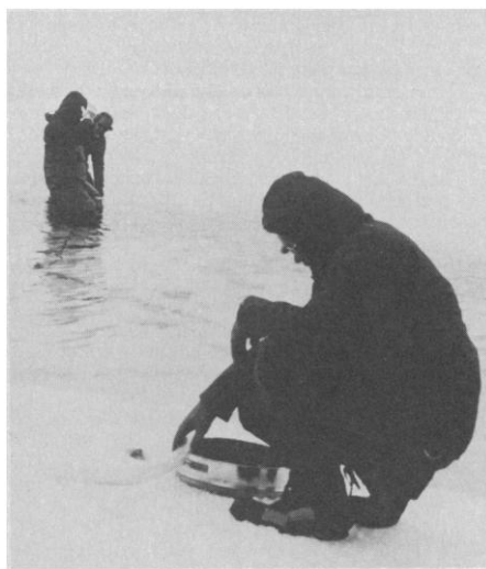
Fig. 1. Collection of dark sediment from a blue ice lake. Particles are vacuumed off the lake bottom and pumped to a 100- \mu m sieve on the lake shore.
