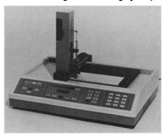
tem. The device is microprocessor-controlled; the user selects volume, band length, and location of each sample. The Linomat IV is useful for preparative work and quantitative analysis. Sample application accuracy and reproducibility exceed 1.0 percent. CA-MAG Scientific. Circle 573.
