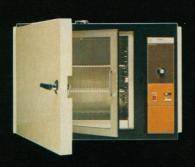
Some like it with forced air. And some like it with gravity. So most units are available in your choice of forcedor gravity-convection airflow patterns. Some even like it without air. Meet the Isotemp Vacuum Oven. It produces temperature from ambient to 280°C in a vacuum of 101.3kPa (30"Hg). Perfect for drying, curing, moisture testing, desiccating and annealing.
