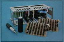
Expandable Card Cage with Boards and Independent Readerhead.
