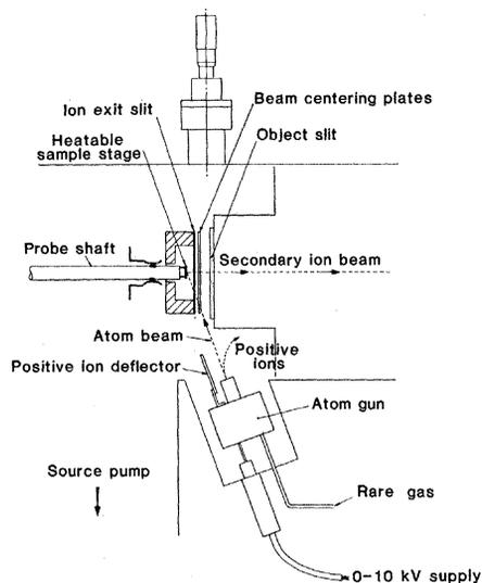
Fig. 1. Diagram of fast atom bombardment ion source. The secondary ion beam provides the mass spectrum. [Courtesy of VG Analytical, Altrincham, England]
