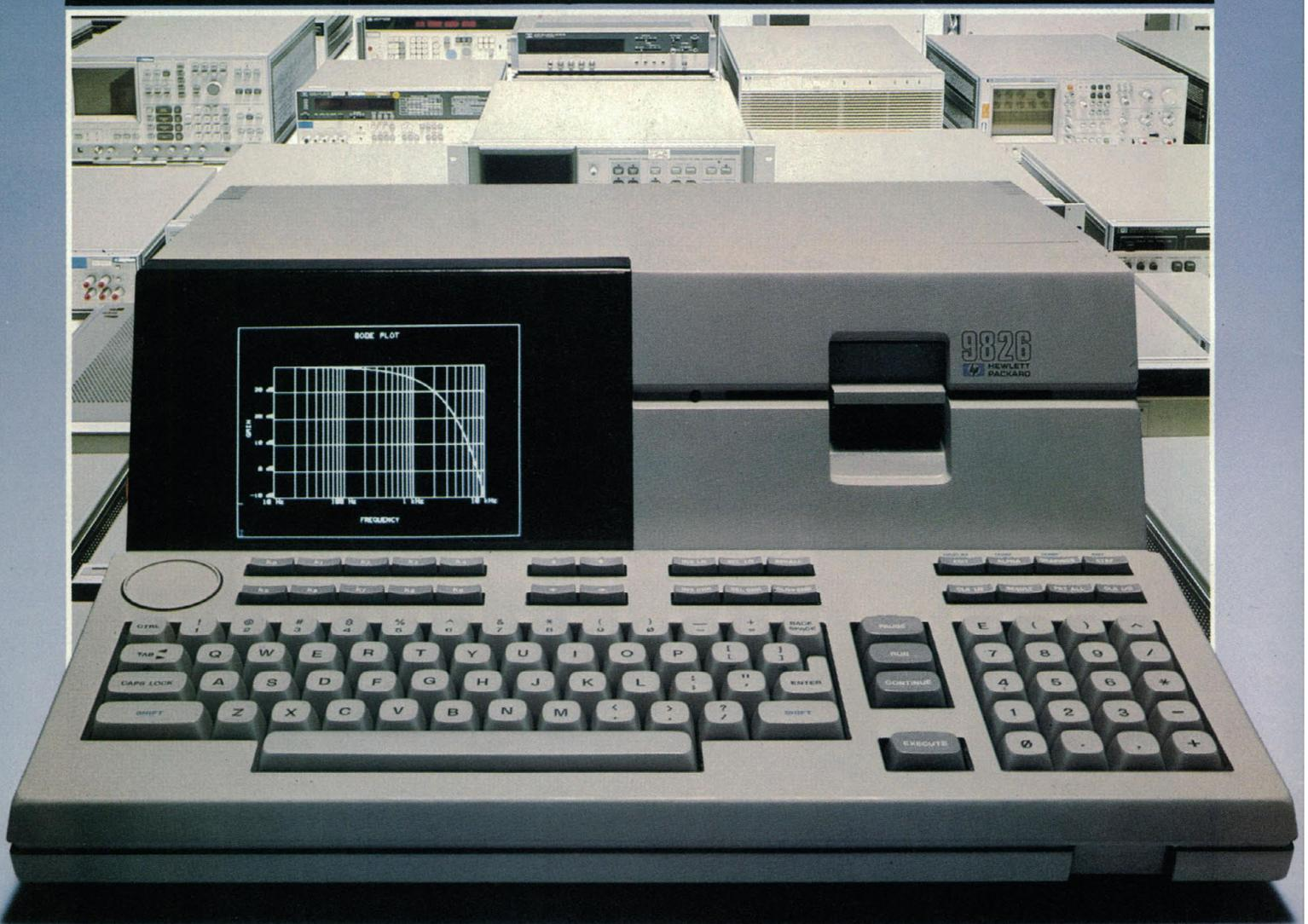
If you're building an automated test system, you've got hundreds of instruments and six interfaces to choose from. And when you try to put it all together, you're in for some long nights in the lab. Unless you use a controller that's been designed just for the job. The HP 9826.
