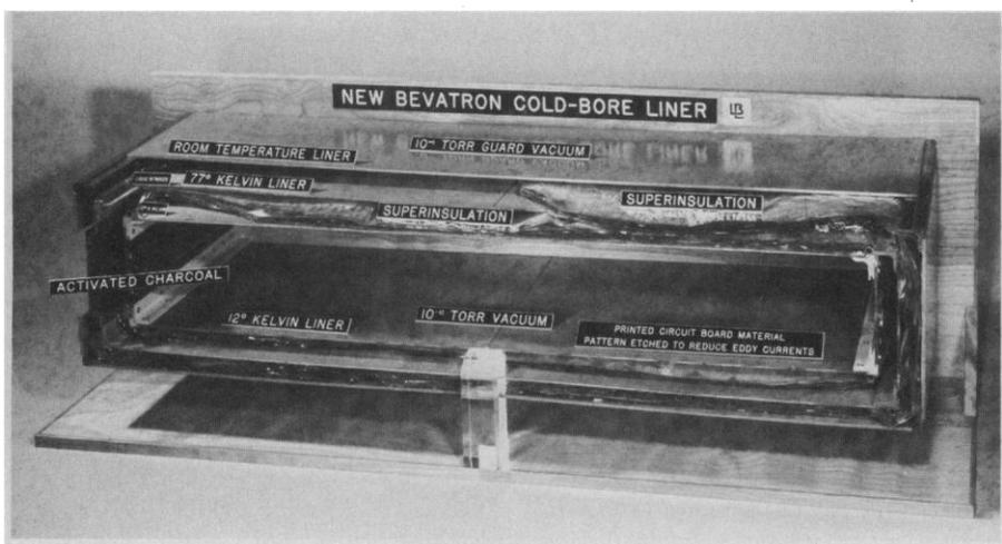
Fig. 2. Cross section model of the new Bevatron cold-bore liner showing the various components.
