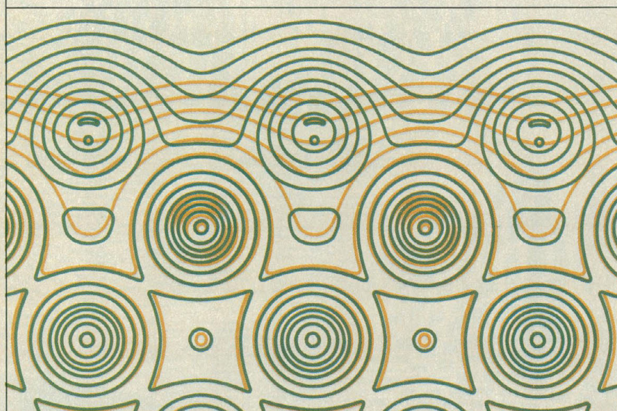
Figure 2: Two electron density contour maps of the cross-section of a Cu(100) surface. One map shows a clean copper surface (tan); the other shows a nitrogen-covered copper surface (green).
