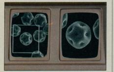
spread and service life are greatly improved compared to conventional LaB<sub>6</sub> or tungsten filament sources. This source operates with an accelerating voltage of up to 30 kV and allows a guaranteed resolving power of 20Å. Magnification of  $20 \sim 300,000X$ .
