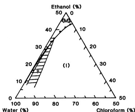
Fig. 1 (left). Diagram showing the solubility of chloroform in the ethanol-water mixture. Chloroform was miscible (M) in the region above the solid line and immiscible (I) in the region below the solid line. Acceptable spherical crystallization occurred in the shaded region. Fig. 2 (right). Micrographs of spherically agglomerated crystals (a) and primary crystals without spherical crystallization (b). Scale bars represent 10 mm in (a) and 200  $\mu$ m in (b).
