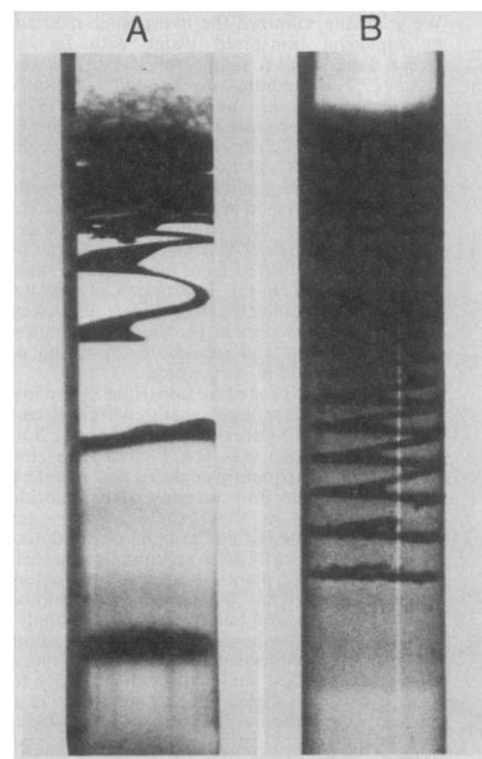
Fig. 3. (A) Spiral band of  $Mg(OH)_2$  after 4 days. Initial electrolyte solutions: 5.5M  $NH_4OH$  (upper portion of tube) and 0.37M  $MgSO_4$  in 8 percent gelatin (lower portion of tube). (B) Spiral band of  $Ag_2Cr_2O_7$  after 1 day. Initial electrolyte solutions: 0.92M  $AgNO_3$  (upper portion) and 6.8 mM  $K_2Cr_2O_7$  in 5 percent gelatin (lower portion). Inner diameter of tubes, 5 mm.
