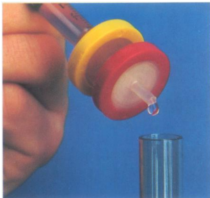
Syringe Filters used in tandem for prefiltration and final filtration.
