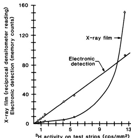
Fig. 1. Comparison of x-ray film and electronic autofluorography of  $^3\text{H}$ -labeled calibration strips of gels containing the scintillant PPO. Exposures for the x-ray film were 48 hours at 23°C and for the electronic detection 34 minutes (sum of 17 2-minute exposures). The autofluorography was carried out by E. P. Lester.
