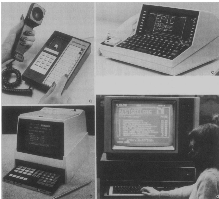
Fig. 5. Examples of increasingly intelligent terminals, made possible by the declining cost of digital electronics. (a) Users can automatically dial any of 12 prerecorded phone numbers by pushing one button on the microcomputer-based Touch-a-matic series telephone. (b) Residential energy management terminal, currently undergoing trial in North Carolina, lets users monitor and control home energy usage. (c) Experimental "teleterminal" with controls whose functions change as the display is changed. (d) Viewtron electronic home information system terminal, currently undergoing trial in Florida.
