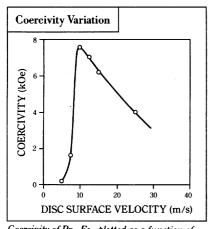
Coercivity of Pr<sub>0.4</sub> Fe<sub>06</sub> plotted as a function of disc surface velocity.
