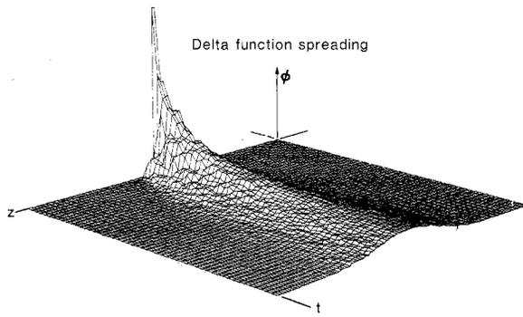
Fig. 2. Development of  $\phi$  as a function of time as a result of random mixing layers simulated on a computer. The initial  $\phi$  is a delta function.
