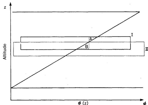
Fig. 1. Mechanism of transport perpendicular to turbulent mixing layers in a stratified fluid. The symbol  $\phi$  denotes pollutant concentration or mixing ratio.
