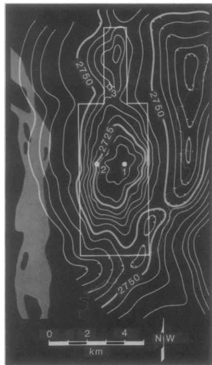
Fig. 7. The same geologic horizon as in Fig. 4 contoured from a three-dimensional seismic survey conducted over the outlined area. This map shows the true structure of the target horizon and that well 3 was drilled on a structural low.
