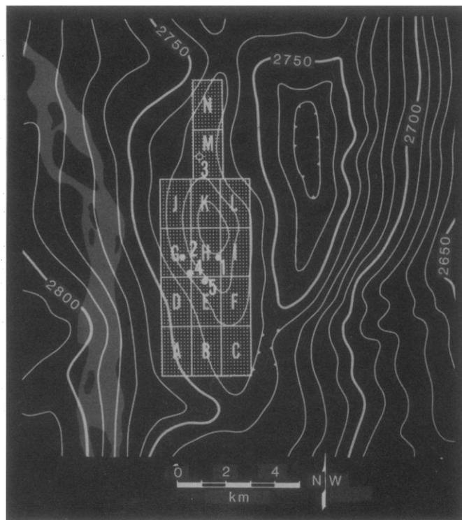
Fig. 4 (left). Contour map of a producing horizon based on seven two-dimensional seismic profiles. Wells 1 and 2 were successful, but well 3 was dry. Fig. 5 (right). Field layout for recording the three-dimensional seismic data. Sources and receivers were located around the perimeter of rectangles A through N. Seismic traces were referenced to the locations by dots inside the area surveyed.
