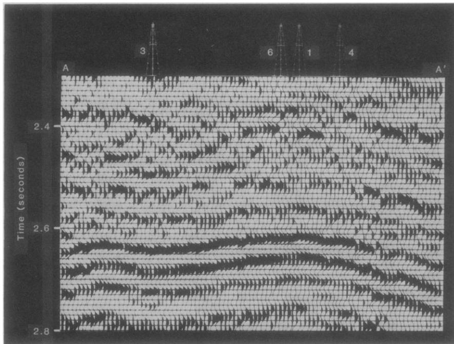
Fig. 6. This three-dimensional migrated section of a traverse assembled through several wells shows that well 3 is located between two structures.
