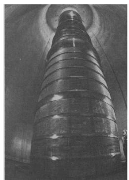
**New Accelerator Dedicated** The Holifield Heavy Ion Research Facility at the Oak Ridge National Laboratory includes a 25-million-volt tandem Van de Graaff (electrostatic) accelerator for nuclei having atomic masses from 12 (carbon) to 160 (terbium).
