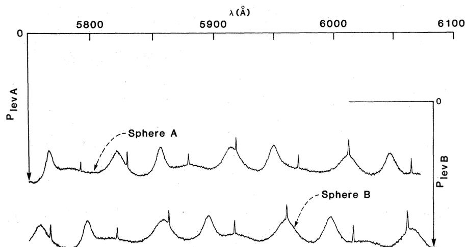
Fig. 3. Resonant behavior of light forces on dielectric spheres. The spectra show the variation with wavelength of  $P_{levA}$  and  $P_{levB}$ , the power needed to levitate oil drops A and B, which have index of refraction  $n = 1.47$  and slightly different diameters ( $\sim 10 \mu\text{m}$ ). The resonances of sphere A are shifted  $\sim 50 \text{ \AA}$  higher in wavelength than the corresponding ones in sphere B.
