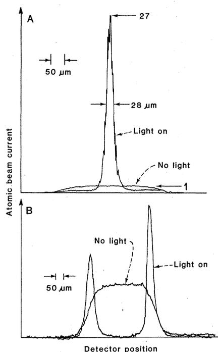
Fig. 7. (A) Focusing of an atomic beam by light tuned below resonance. (B) Defocusing of an atomic beam by light tuned above resonance.
