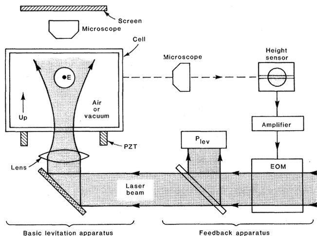
Fig. 2 (right). Basic apparatus for optically levitating dielectric spheres and feedback stabilization apparatus for levitating in vacuum and measuring forces. Abbreviations: PZT, piezoelectric ceramic shaker; EOM, electrooptic modulator.
