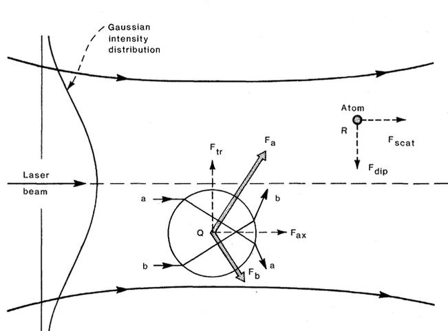
Fig. 1 (left). Optical forces on a dielectric sphere and an atom in a TEM<sub>00</sub> mode Gaussian laser beam.
