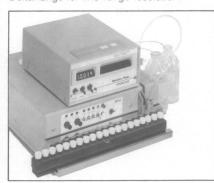
Density meters. Unique use of electromagnetic excitation of the sample tube makes every Mettler/Paar Digital Density Meter a breeze to use. Accuracy is
