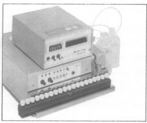
Density meters. Unique use of electromagnetic excitation of the sample tube makes every Mettler/Paar Digital Density Meter a breeze to use. Accuracy is unaffected by viscosity or volatility or surface tension of the specimen. Digital results in seconds for density, specific gravity or concentration. Anyone can use
