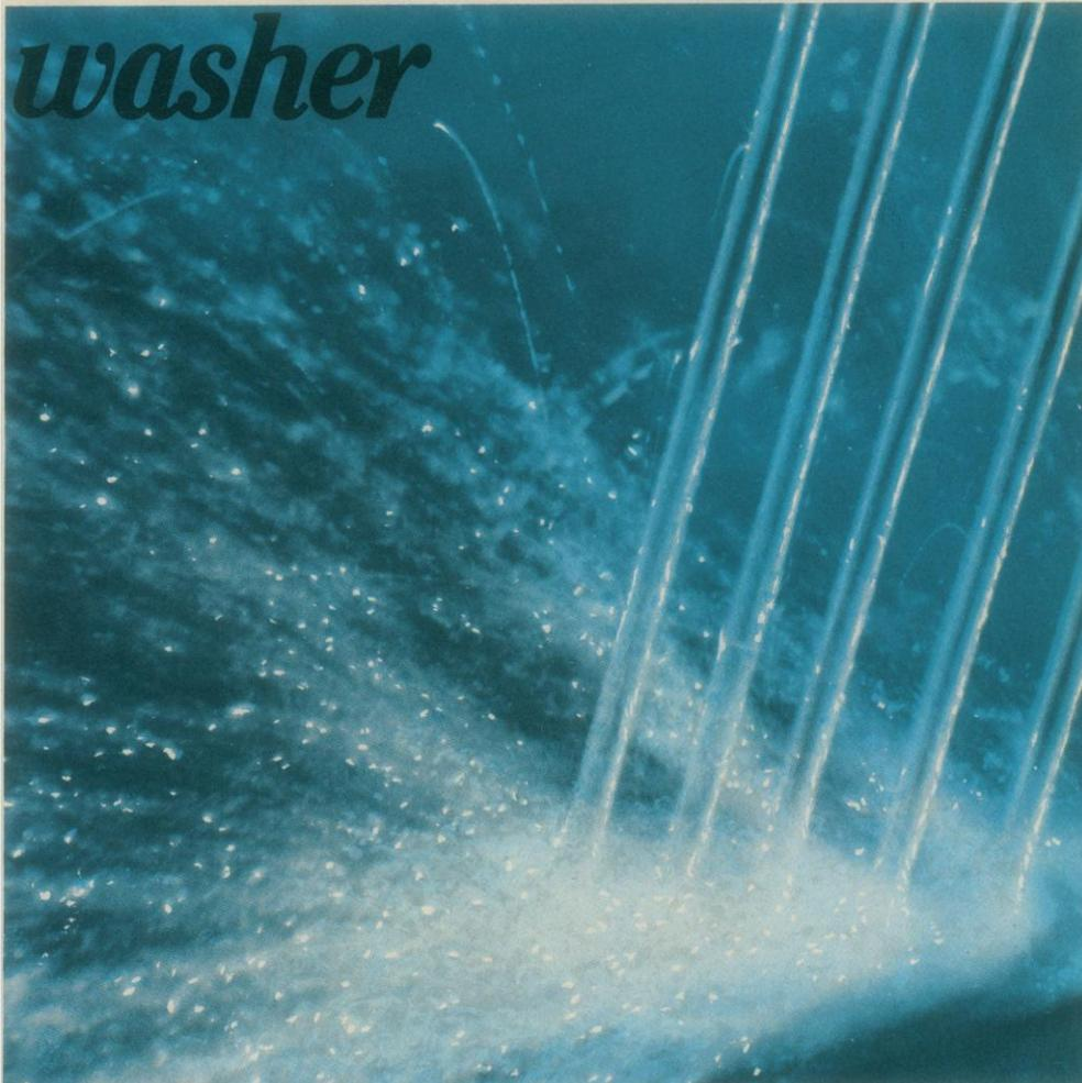
*Most industrial washers are adapted from the home dishwasher. The same plumbing and the same nozzles are used for the pre-wash, detergent and rinse cycles. Cross contamination is unavoidable from one cycle to another.*
