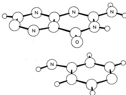
Fig. 3. Intermolecular stacking arrangement of the pteridine and phenyl rings in the folic acid crystal structure. Perpendicular separation of the two ring planes is 3.28 Å.
