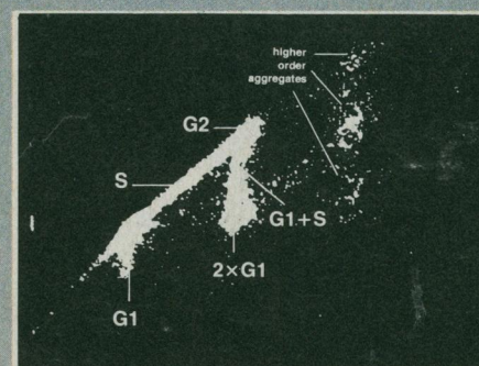
2. Cytogram of somewhat clumped Erlich ascites tumor cells, stained for DNA with ethidium bromide. Correlation of pulse area measurement (X) with pulse height (Y) permits distinguishing G2 cells from 2 x G1 aggregates.
