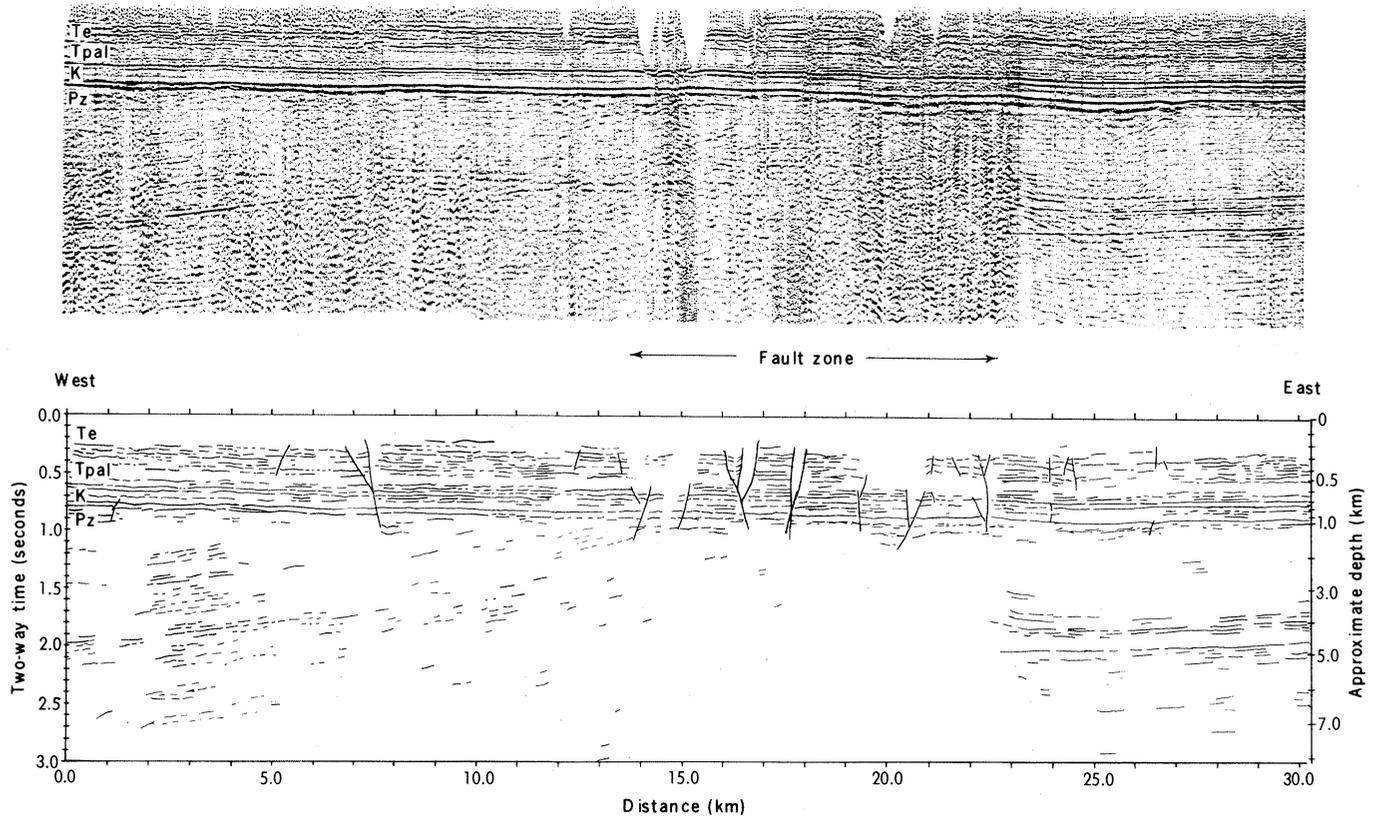
Fig. 4. Part of profile D-1 and a corresponding interpretative line drawing. Ages of units are as indicated in Fig. 3. Note that the depth scale is nonlinear.
