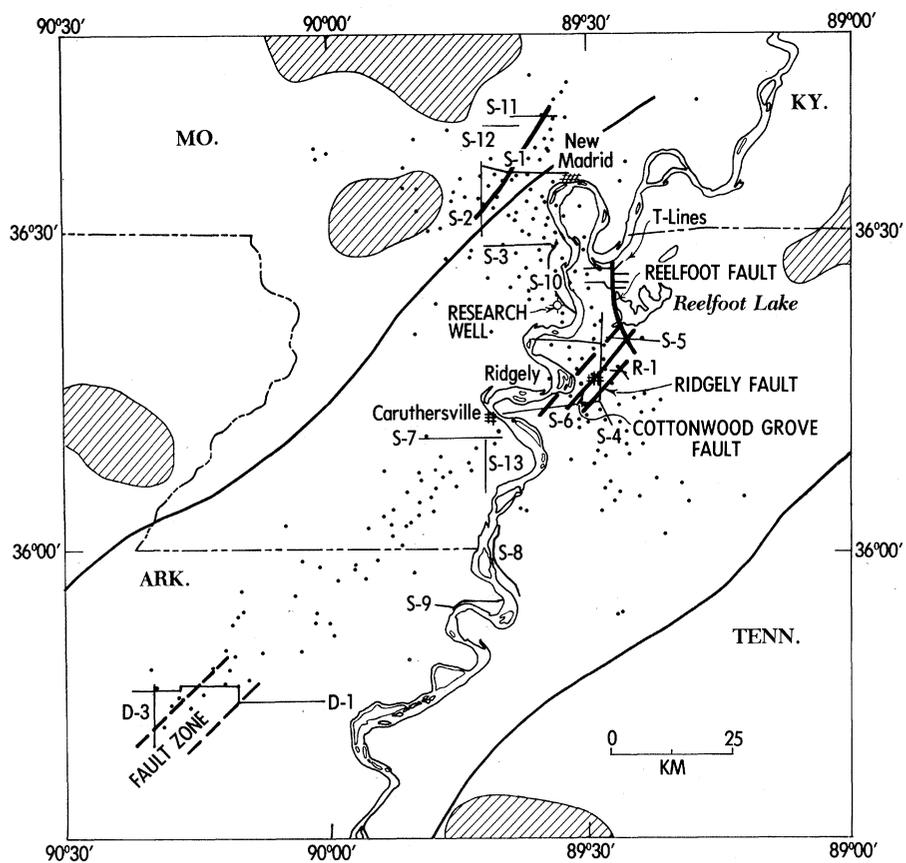
Fig. 2. Enlargement of part of Fig. 1 showing earthquake epicenters (dots) (31), the locations of the seismic reflection profiles, and principal faults inferred from the data.
