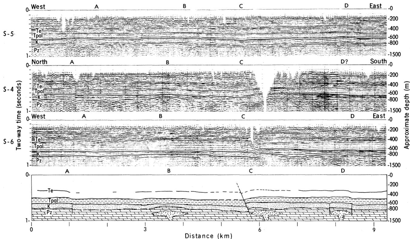
Fig. 3. Part of profiles S-5, S-4, and S-6, and (bottom) an interpretative, oblique cross section of the fault system. The main features are A, northwest boundary fault; B, Cenozoic intrusion and overlying, arched reflectors; C, Cottonwood Grove fault; and D, possible intrusion. Geologic ages of rocks are indicated as *Te*, Eocene; *Tpal*, Paleocene; *K*, Cretaceous; and *Pz*, Paleozoic. Note that the depth scale is nonlinear.
