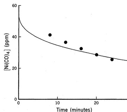
Fig. 1. Plot of [Ni(CO)<sub>4</sub>] versus time at a calculated initial [Ni(CO)<sub>4</sub>] of 52.5 ppm. The points are data obtained by syringe injection into a stirred 5-liter flask. The curve is the calculated decomposition for a homogeneous mixture of Ni(CO)<sub>4</sub> in air at the same initial [Ni(CO)<sub>4</sub>], based on the rate constants derived herein.
