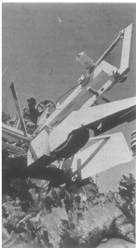
A prototype lettuce harvester developed by USDA engineers in California. In this early version, an x-ray device just behind the lifted wheel measures the density of each lettuce head and activates a blade, cutting only mature plants. [USDA photo]
