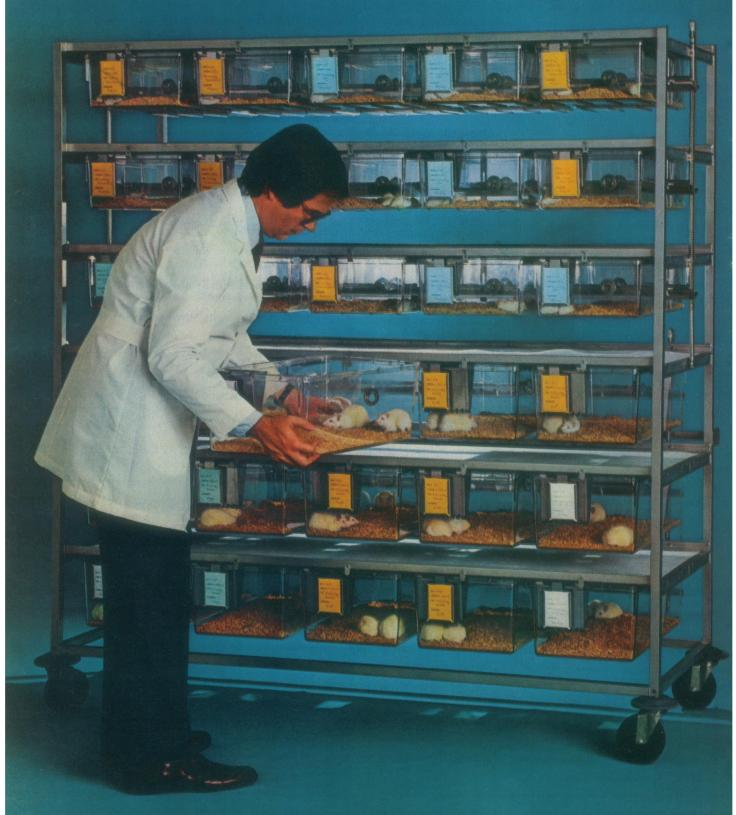
\*Please note that the unit shown above is merely a demonstration model assembled to show that the rack can accommodate a single large cage in each position . . . or, alternatively, two small ones.
