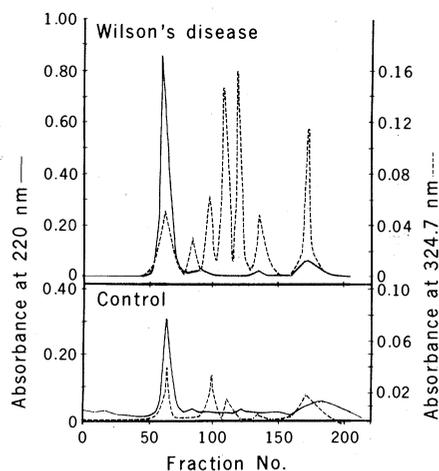
Fig. 1. Sephadex G-50 column chromatography of cell lysates. The gels were equilibrated with 0.02M tris-acetate (pH 8.6), and proteins were eluted at a flow rate of 25 ml/hour. Proteins were monitored with absorbance at 220 nm. Copper was monitored by flameless atomic absorption spectroscopy with absorbance at 324.7 nm.
