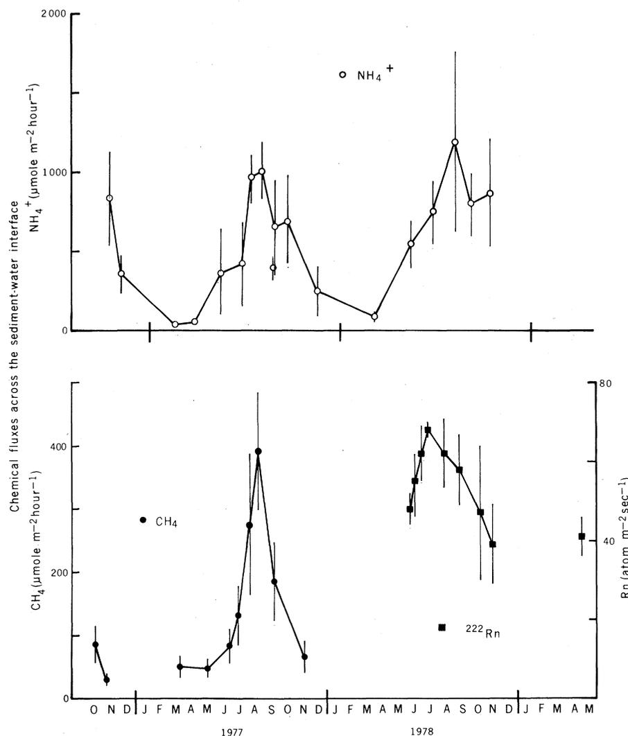
Fig. 2. Seasonal variations in chemical fluxes across the sediment-water interface observed in Cape Lookout Bight, North Carolina. In situ benthic chambers were used. Error bars ( $1\sigma$ , where  $\sigma$  is the theoretical standard deviation) are calculated from multiple chamber emplacements.
