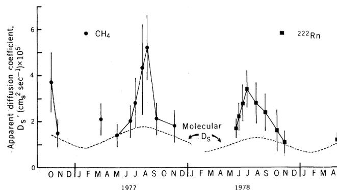
Fig. 3. Seasonal variations in the apparent sediment diffusivities ( $D_s'$ ) calculated from in situ  $\text{CH}_4$  and  $^{222}\text{Rn}$  flux measurements in benthic chambers in Cape Lookout Bight. Theoretical molecular sediment diffusivities ( $D_s$ ) for  $\text{CH}_4$  and  $^{222}\text{Rn}$  are also shown. Error bars =  $\pm 1\sigma$ .
