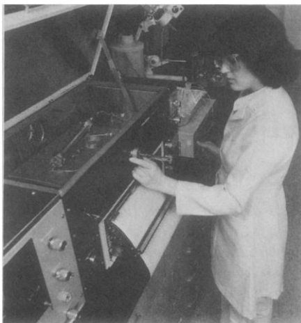
Lid of oven chamber on Du Pont's new HPPLC system is raised to show the column in place. Sample is injected through the port above the operator's hand. [Source: Du Pont]
