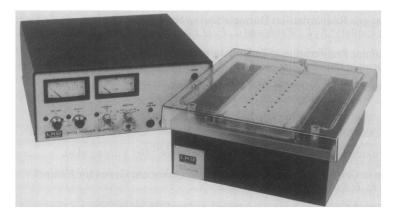
That's how easy it is with LKB's Multiphor® unit. And duration of the runs is also short: the precisely engineered all-glass cooling stage means that you can apply higher power for faster runs higher field strengths for sharper resolution. With the Multiphor unit and LKB's power supply you can do up to 48 samples in less than two hours!
