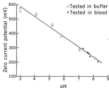
Fig. 1. Calibration curve of a Pd-PdO pH electrode in buffer solutions and whole blood at 310 K. The potential was measured versus an Ag-AgCl electrode.
