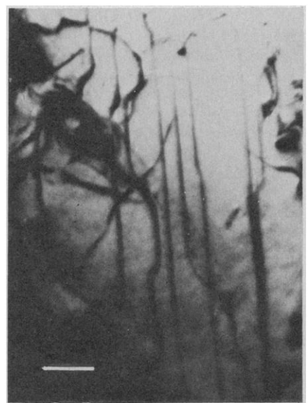
Fig. 4. Straight dislocations along [\bar{1}10] in the (111) plane of ringwoodite; scale bar, 0.1 \mu\text{m} .
