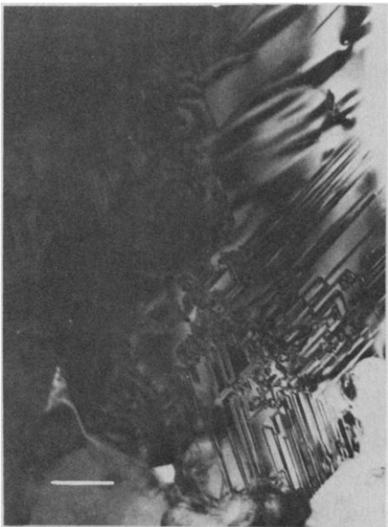
Fig. 2. Planar defects in a ringwoodite grain; scale bar, 0.2 \mu\text{m} .
