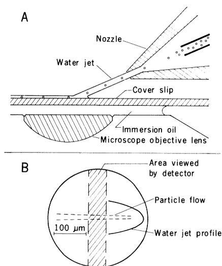
**Fig. 1.** The essential part of the flow system. (A) A collimated beam of cells in a pressurized water jet, formed by hydrodynamic focusing, hits a glass cover slip at low angle to form a flat, laminar stream with the cells confined to a narrow sector. The cover slip is viewed by means of an inverted fluorescence microscope with incident illumination. (B) The flow as it appears in the microscope. The shaded area indicates the section viewed by the fluorescence detector.
