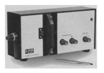
Sensitivity is increased up to 200x for proteins when you monitor at 206 nm with LKB's new Uvicord® S UV-monitor. This unique instrument will detect non-aromatic peptides, polysaccharides, nucleotides, lipids and steroids as well as proteins. And, naturally, you can also monitor at 254 or 280 nm.
