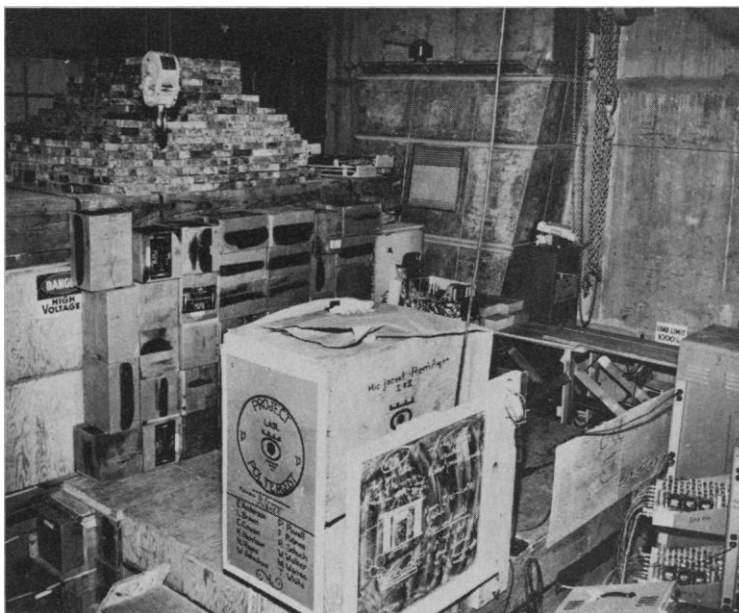
Fig. 2 (left). First large ( 0.3 \text{ m}^3 ) liquid scintillation detector in shield. The liquid was viewed by 90 2-inch photomultiplier tubes. Before the development of this detector a 0.02\text{-m}^3 volume was considered large. Fig. 3 (right). Shield configuration. The note on the blackboard indicates that we were within a factor of 75 of the required sensitivity. The members of the group for the Hanford phase of the search are listed on the "Project Poltergeist" sign.
