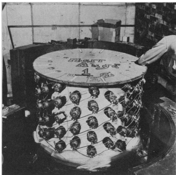
Fig. 2 (left). First large ( 0.3 \text{ m}^3 ) liquid scintillation detector in shield. The liquid was viewed by 90 2-inch photomultiplier tubes. Before the development of this detector a 0.02\text{-m}^3 volume was considered large. Fig. 3 (right). Shield configuration. The note on the blackboard indicates that we were within a factor of 75 of the required sensitivity. The members of the group for the Hanford phase of the search are listed on the "Project Poltergeist" sign.
