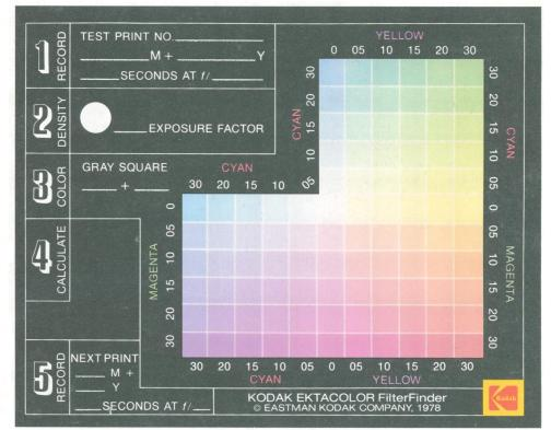
It's a black mask of film—the Kodak Ektacolor FilterFinder—bearing one clear hole and 96 precise tints of color. It works with a gray card that you include in a test shot made at the scene on the same roll of film. When you begin your printing, you place the FilterFinder on the enlarging easel over the image of the gray card to make a test print. From the image of the clear hole on the processed test print, with the use of this Locator ▼
