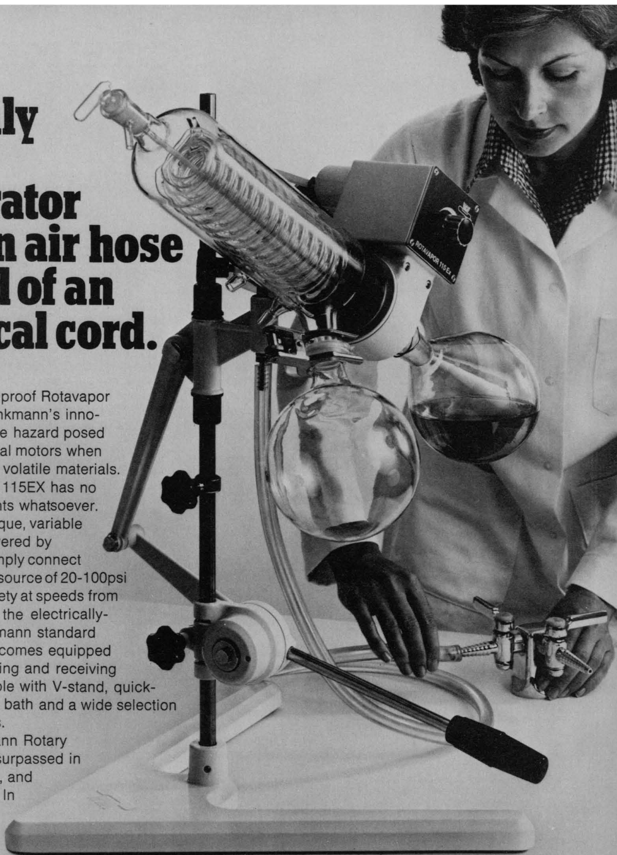
ROTAVAPOR R-175EX For 20-liter volumes. Explosion-proof motor.
