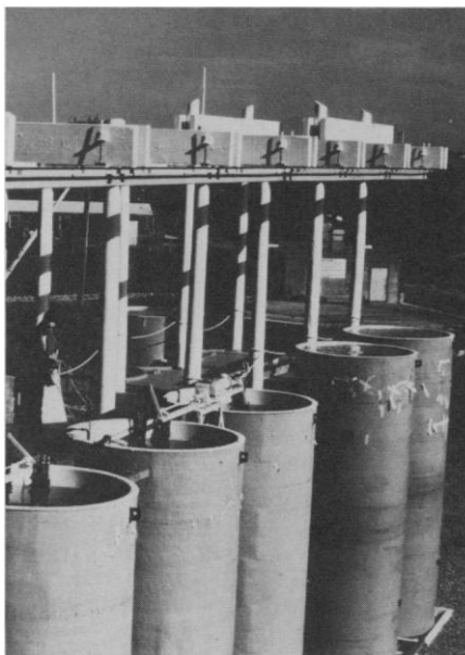
Fig. 1. Controlled ecosystem enclosures at the Marine Ecosystem Research Laboratory (MERL), Narragansett, R.I. Motor and shaft above tank tops operate stirrer within the water column to simulate the natural mixing of an estuary.
