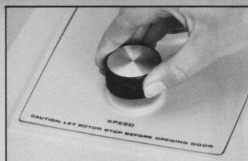
Operation is quite simple. A single knob adjusts air pressure to control rotor speed. The only other control is the timer.
