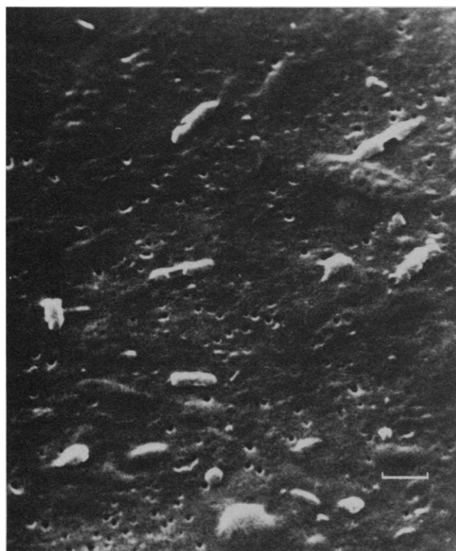
Fig. 1 (left). A scanning electron micrograph photograph of organic particles retained on a 0.1- \mu\text{m} Nuclepore filter from the soil solution collected below the A2 horizon of a Podzol soil from Findley Lake, Washington. Scale bar, 1 \mu\text{m} ( \times 5400 ). Fig. 2 (right). A scanning electron micrograph photograph of silicate particles retained on a
