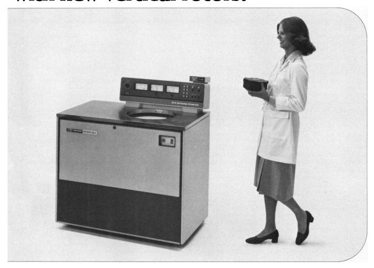
The oil turbine drive also eliminates the maintenance and replacement of gears, belts and brushes. The many other features of OTD centrifuges include trouble-free self-contained cooling system; precise, wide-range temperature control; and automatic and manual vacuum pumping system.
