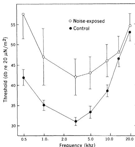
Fig. 1. Mean ( $\pm$  S.E.) 1.0  $\mu\text{V}$  threshold versus frequency for six 45-day-old control animals and nine 45-day-old animals exposed to noise at 40 days of age.
