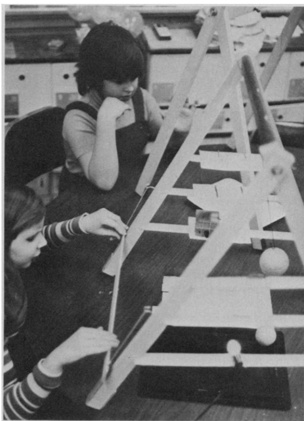
A blind child and her lab partner set up pendulum apparatus. Note the light sensor and light bulb opposite it.
