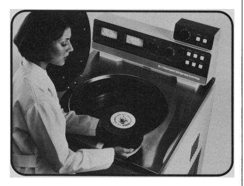
The Sorvall® RC-5 refrigerated superspeed centrifuge with a Rate Controller is ideal for density gradient work. The soft start and soft stop characteristics of the Rate Controller prevent mixing of the gradient at speeds between 0 and 1,000 rpm
